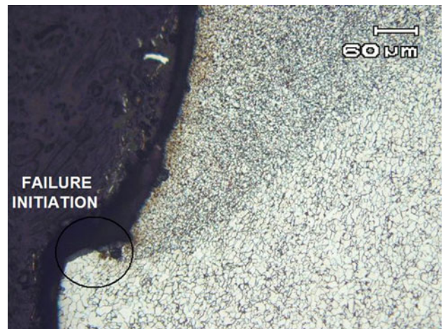
Fig. 6 Metallography of the region of failure initiation showing the location of the fatigue crack nucleation site. Magnification: 200×. Reagent: NITAL 2%
